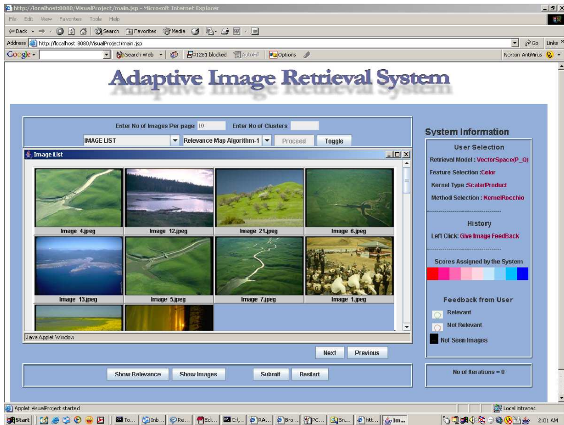
Figure 2. List view. This image displays the interface of the AIRS. The "System Information" box on the right presents a history of the system. The result list is displayed by using the selected view type in the center area, which is surrounded by buttons for different inputs.
